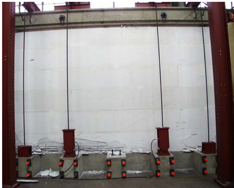
Figure 5.23 Crushing of the compressive toes of Shear Wall Specimen 1
