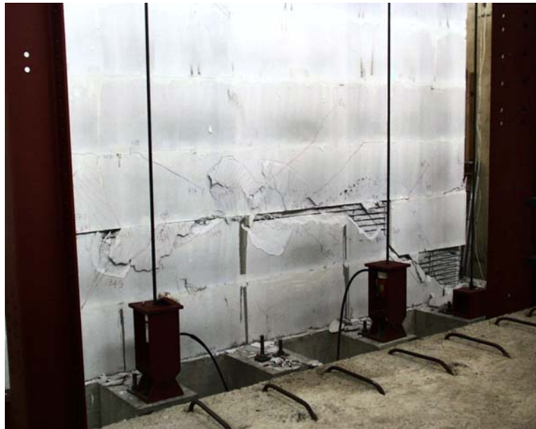
Figure 5.27 Elevation view of Shear Wall Specimen 4 at the end of the test
