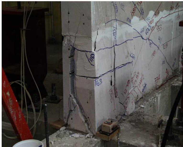
Figure 6.27 North compressive toe of Shear Wall Specimen 13 at the end of the test
