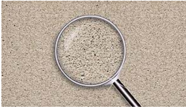
Figure 2.1 Cellular structure of AAC
