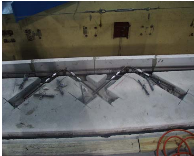
Figure 142: Picture of diagonal reinforcement across the joint parallel to the direction of load in Two-story Assemblage Specimen
