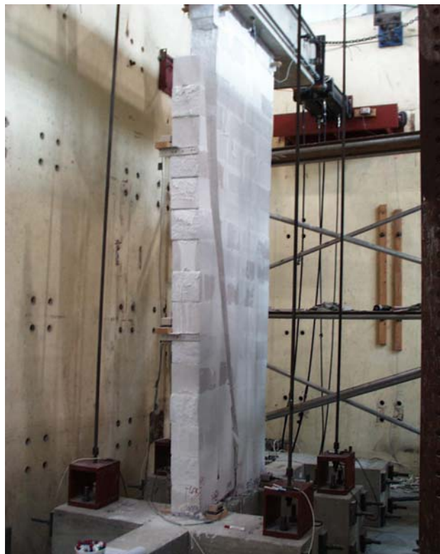
Figure 5.29 Elevation view of Shear Wall Specimen 11 at the end of the test
